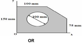
7 Calculate the moment of inertia of shaded area shown in the following figure below, with respect to the centroidal axes parallel to x axes and all the units are in mm.
