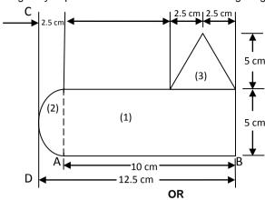
A thin plate of 6 mm thickness is cut and machine component is made from the plate as shown in figure given below. Assuming the density of steel as 7850 kg/m³, calculate the mass moment of inertia about z-axis as shown in figure given below.
