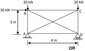
11 A braced cantilever truss is loaded as shown in figure below. All the members are of the same material and have the same cross sectional area. Find the axial force in the member AD by strain energy method.
