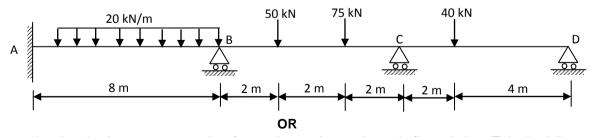
11 Determine the plastic moment capacity of a continuous beam shown in figure below. Take  $\lambda = 1.7$ .
