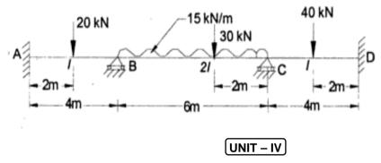
Analyze the beam given in below, by flexibility method. Take EI as constant. The beam undergoes settlement of supports B and C by 10/EI and 5/EI respectively. Draw the bending moment diagram.
