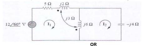
3 Determine the currents  $I_1$  and  $I_2$  for the circuit shown in figure below.
