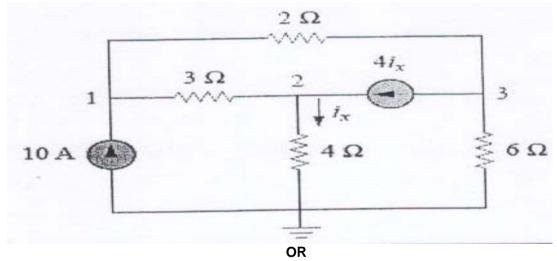
7 Using Mesh analysis determine i<sub>1</sub>, i<sub>2</sub>, i<sub>3</sub> for the circuit shown in figure below.
