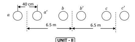
4 Determine the A, B, C, D constants for a three phase 50 Hz transmission line, 250 km long having the following distributed parameters  $I = 1.15 \times 10^{-3}$  H/km,  $c = 7.8 \times 10^{-9}$  F/m, r = 0.14 ohms/km, g = 0.
