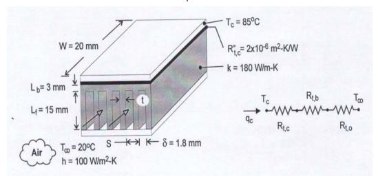
Assumptions: (i) Steady-state. (ii) One-dimensional heat transfer. (iii) Isothermal chip. (iv) Negligible heat transfer from top surface of chip. (v) Negligible temperature rise for air flow. (vi) Uniform convection coefficient associated with air flow through channels and over outer surface of heat sink. (vii) Negligible radiation.
