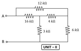
3 Obtain the Thevenin's equivalent circuit at terminals AB of the circuit shown below.
