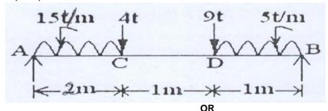
5 Find the shear force at the supports of the beam given below.
