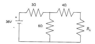
(b) Using Norton's theorem, find the current in the load resistor  ${\cal R}_L$  in the network shown in figure.
