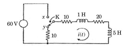
R-L-C circuit is excited by DC voltage source. Find (*b*) Current i(t) using conventional method. The switch is closed at time t = 0. [6]
