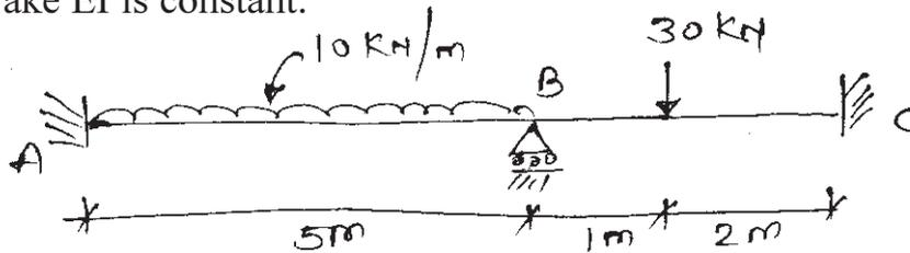
b) Analyse the continuous beam shown in figure using flexibility method & draw the bending moment diagram. [10]
