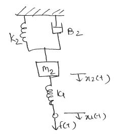
Q5) a) For each of the following system find poles of system, plot them on s plane. Without solving for inverse Laplace transform plot the nature of time response to step i/p in each case.[6]
