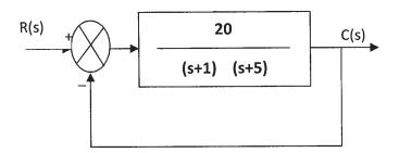
Determine the characteristic equation of the system,  $\omega n$ ,  $\xi$ ,  $\omega d$ , tp, Mp, the time at which the first overshoot occurs, the time period of oscillations and the number of cycles completed before reaching the steady state.
