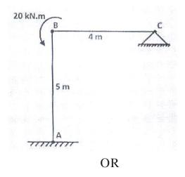
**Q6**) Determine unknown joint displacements at node B of the orthogonal grid as shown in figure. Take  $EI = 1500 \text{ kN.m}^2$  and  $GJ = 700 \text{ kN.m}^2$  [10]
