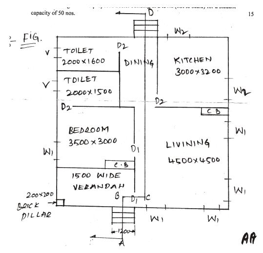
**7.** Draw a line diagram for a proposed hostel building in a town (not to scale) for a student capacity of 50 nos.
