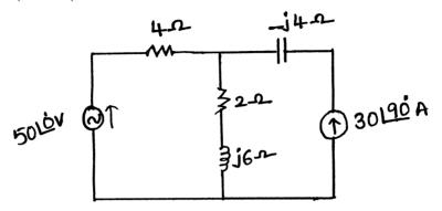
14 Find the voltage drop across the  $2k\Omega$  resistor by using node analysis technique.
