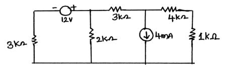
15 (a) Write the mesh current equations in the circuit and determine the currents  $I_1, I_2$
