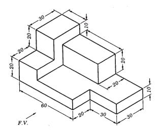
**9.** Draw the isometric view of the object, whose orthographic views are given in the figure below:
